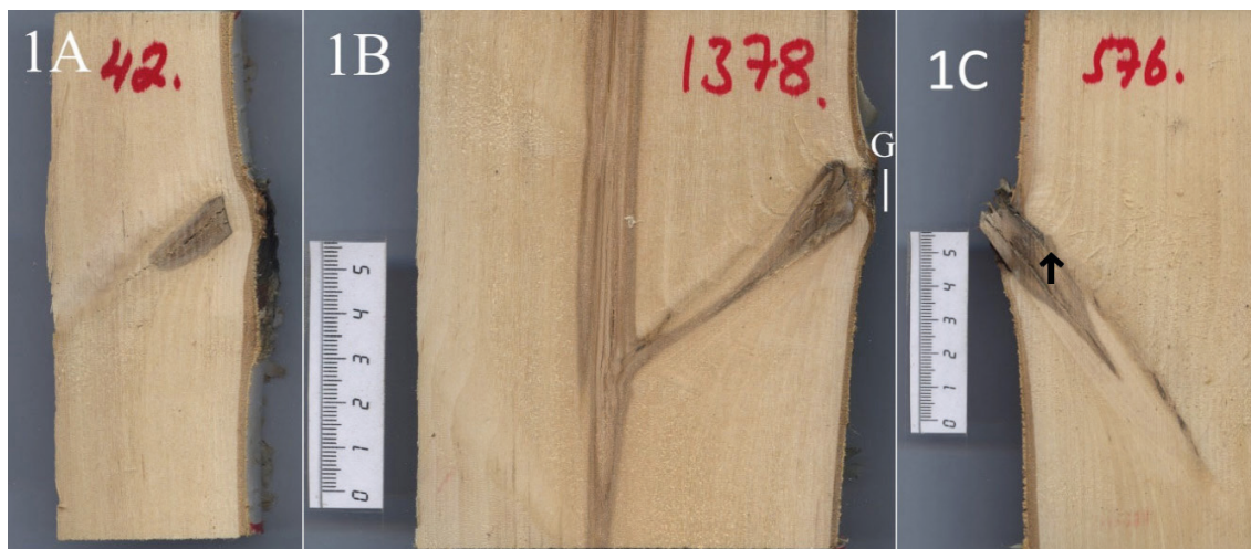
Fig. 1. Three scanned images of study knots: Knot 1A: a 12-mm-thick knot occluded without discolouration (occlusion class 1). The occlusion gap was closed and the occlusion rate was set to 100%. Knot 1B: occlusion started from the up and down sides of a 16-mm-thick knot (class 3). Because the occlusion gap (G) was 7.7 mm long, the occlusion percentage was 52%. Knot 1C: vertical diameter of the knot was 13 mm and the occlusion gap was not measured because no occlusion was observed (class 6). The occlusion rate was set to 0%. A small discolouration in the stemwood (upward \uparrow ) was also detected.
