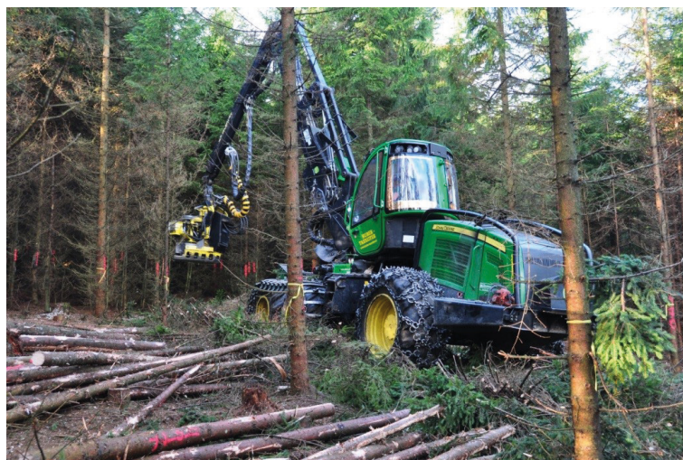
Fig. 4. Harvester John Deere 1170E with H414 harvester head-unit at the thinning operation on the skid trail with already processed logs along the skid trail and the stand to be thinned in front of the harvester.
