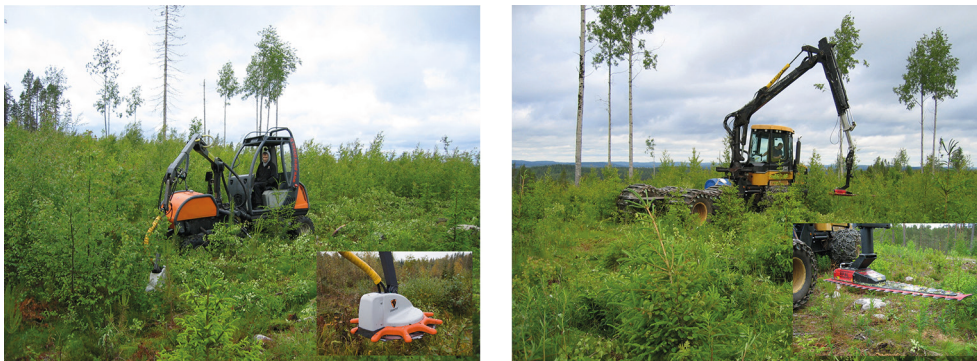
Fig. 1. Machines used in the study: Usewood Tehojätkä small-scale forest machine equipped with UW40-cleaning head (left) and Mense RP6L equipped on the boom of the harvester (right) Photos: Veli-Matti Saarinen and UW40-cleaning head: www.usewood.fi .
