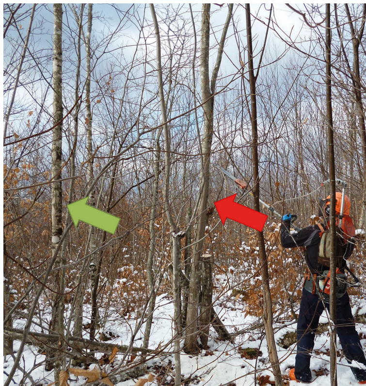
Fig. 1. Worker performing precommercial crop tree release (PCTR) with the Husqvarna 535FBx spacing saw in the study stand. Green arrow points to a maple crop tree while red arrow points to a beech competitor about to be cut.
