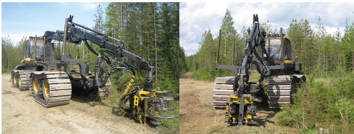
Fig. 1. The studied harwarder consisting of a Ponsse Buffalo Dual forwarder and the Moipu 300 F1 harwarder head. The harvesting of brushwood was based on the dual purpose machine system.
