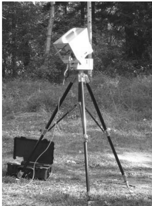
Fig. 4. The laser scan head is mounted on a pan-tilt base permitting bi-directional rotation. It is powered by a battery pack and scanning is controlled remotely through a hand-held device. Data is written to a USB-port on the rear panel of the scan head.
