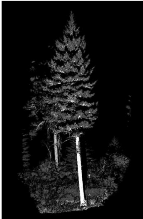
Fig. 5. An original single (unmerged) tree scan as initially visualized. Note that the sample tree in the foreground will be isolated by removing returns from other vegetation in the scene.
