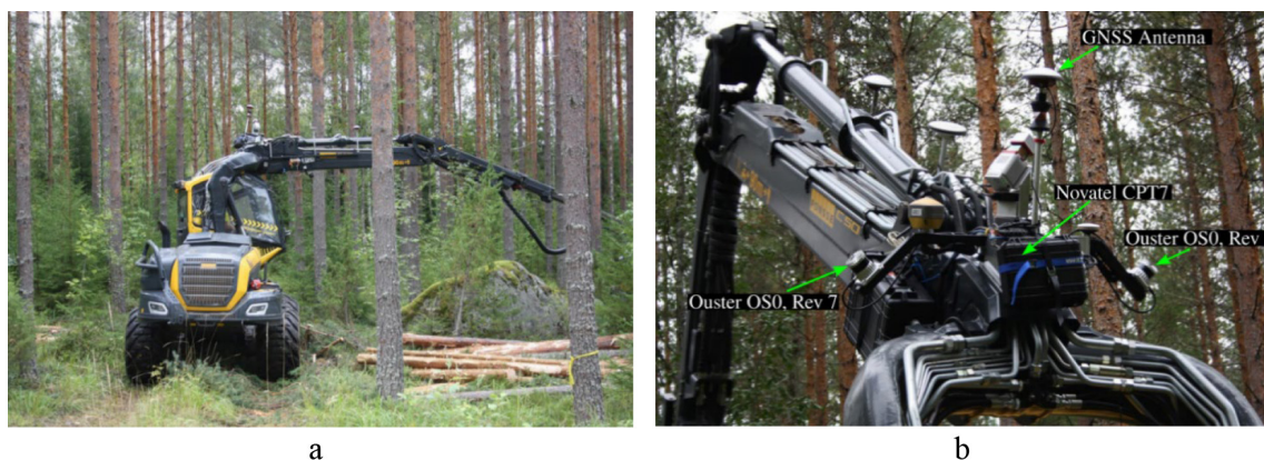
Fig. 1. Study site and the Ponsse Scorpion harvester used for the study (a), and the position of the two Ouster LiDARs, one GNSS antenna, and Novatel CPT7 installed on the boom of the Ponsse harvester (b). The Novatel CPT7 was behind the black box attached to the aluminium frame, not inside the black box.
