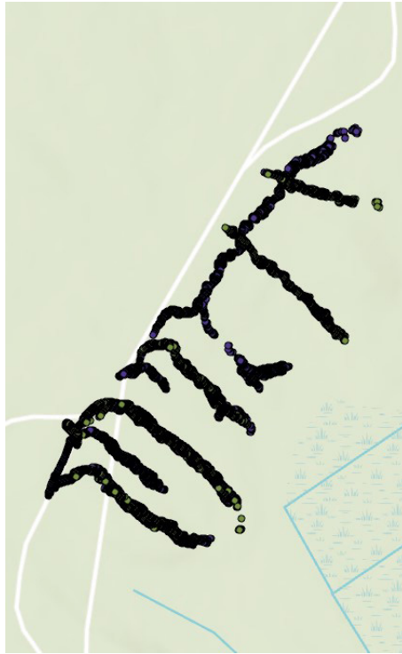
Fig. 4. Harvester trajectory. During the harvesting operations, the trajectory of the harvester was monitored using a robotic total station.
