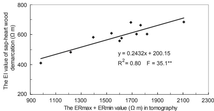
**Fig. 6.** Relationship between the maximum ER plus minimum ER (ERmax + ERmin) values and the corresponding electric resistivity (ER) value of the sapwood-heartwood demarcation (of an incremental core) of the tomographic data (Luanata fir (*Cunninghamia konishii* Hayata),  $n = 11$ ).
