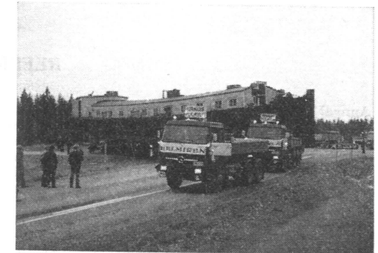
Fig. 3. A house barge being moved by truck from one part of the water system to another.
