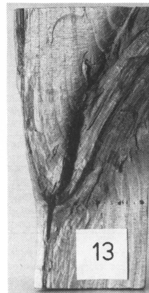
Fig. 5. Thick knot with unclear lower edges, large branch angle, in which the direction of convexity of the knot pith has clearly changed (edge 5 cm).
