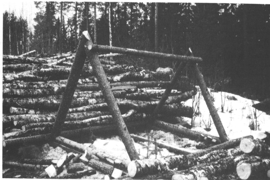
Fig. 3. Triangular frame used in creating cavities in sample piles.
