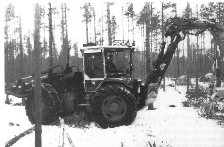
Fig. 2. Huddig 960 backhoe loader with Tufab GS 301 harvester head and an extra dipper attached to the original crane (machine no. 2).
