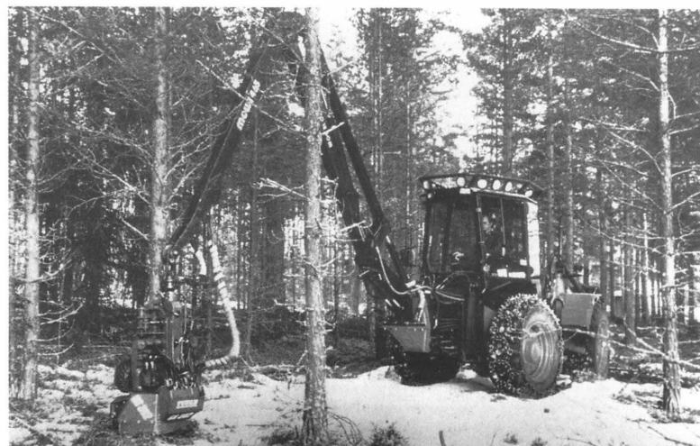
Fig. 3. Huddig 760 M4 backhoe loader with Tufab GS 302 harvester head (machine no. 3). The original crane is replaced by a Mowi 465 parallelogram crane.
