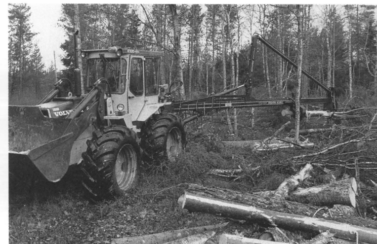
Fig. 1. Volvo 6300 backhoe loader with Skogserik RC 380 P stroke delimiting processor (machine no. 1). Original crane removed.
