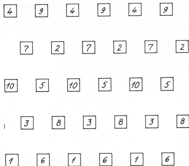
Fig. 2. The principle employed in setting out the survey tracts in Sweden.
