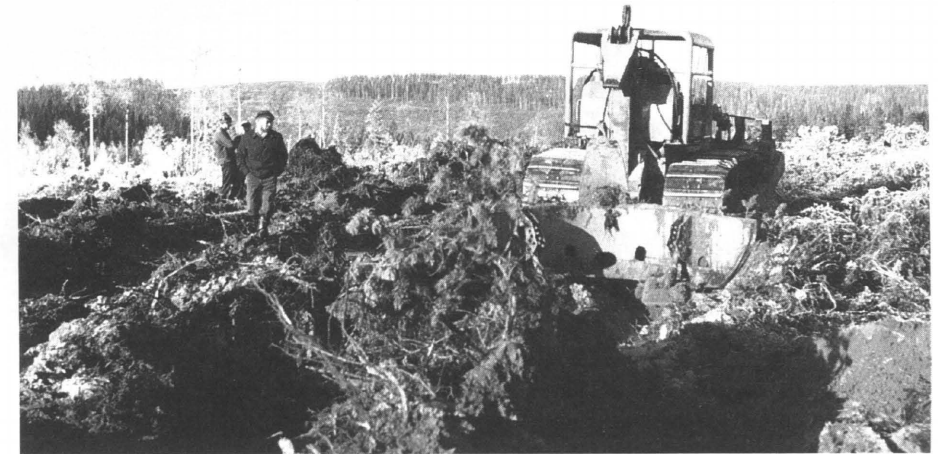
Figure 2. The reforestation plough and the caterpillar tractor used for shoulder ploughing and cross-directional ploughing.
