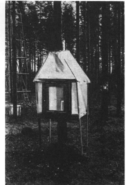
Figure 8. Plastic chamber in the Metsä-Saramäki experimental stand. The girth bands are above, under, and in the chamber. Photo June 8, 1964.
