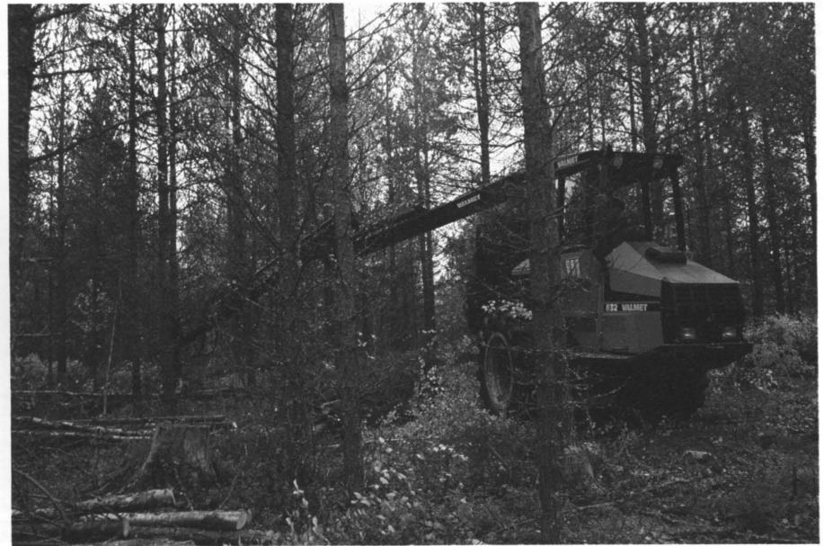
Figure 19. A medium-sized forwarder, equipped with a long-reach crane, is the principal solution for off-road transport of timber. Valmet 832 forwarder (Photo H. Kalaja).
