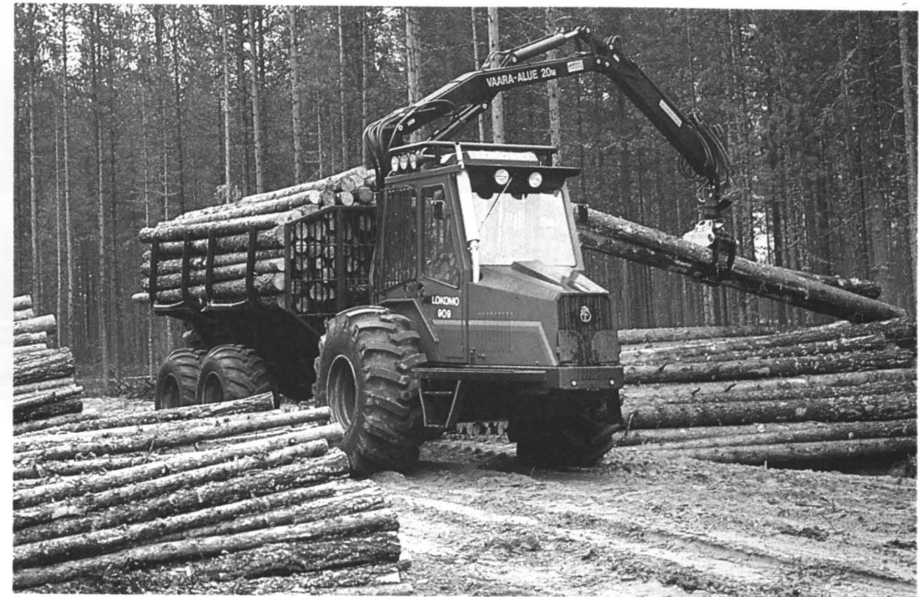
Figure 12. In the log-length method, a load-carrying tractor sorts the timber according to assortment at the landing site. Lokomo 909 forwarder (Photo FMG Lokomo Forest Oy).
