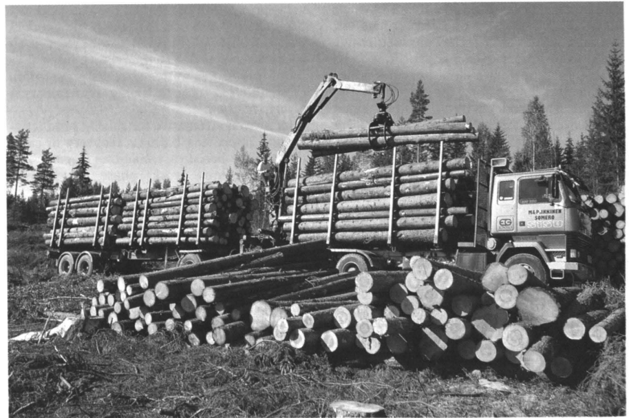
Figure 20. A three-axle truck, equipped with a three-axle full-trailer and a detachable grapple crane, is the most common combination for long-distance transport of timber. Sisu SM 320 timber truck, Fiskars MZ crane, and Jyki trailer (Photo H. Kalaja).
