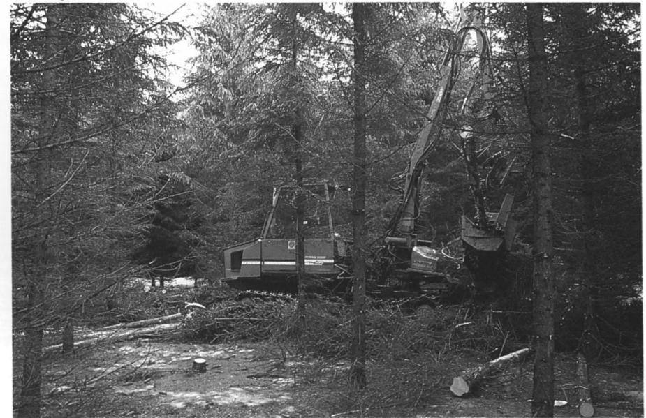
Figure 28. Light harvesters are capable of operating in young thinning stands. Nokka Joker double-grip harvester, equipped with Nokka felling head and Hakki processor (Photo Erkki Oksanen).
