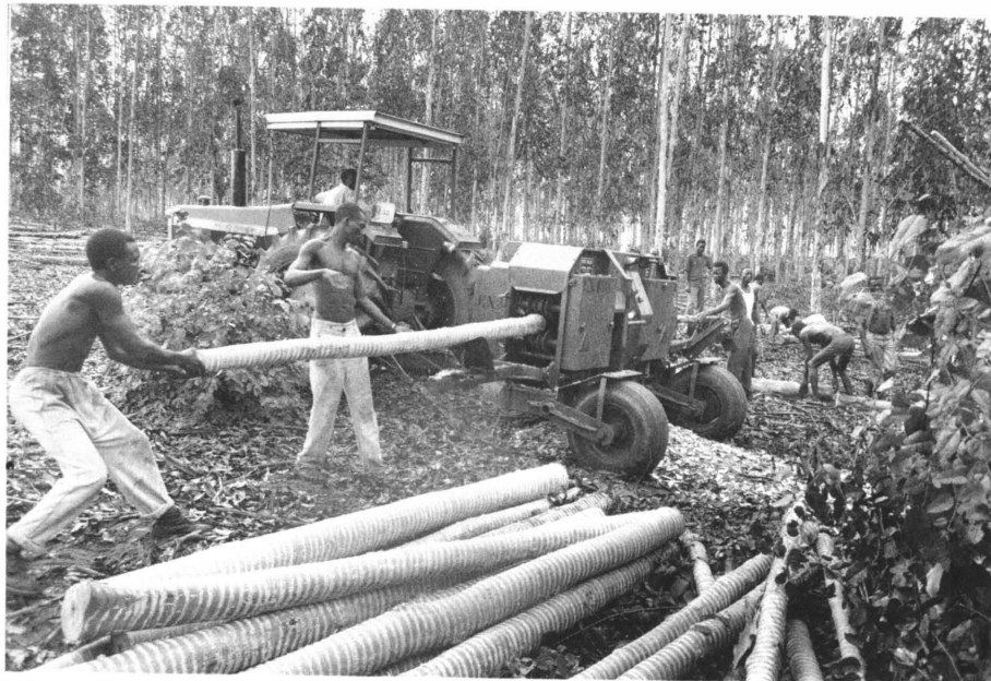
Figure 26. In Finland debarking of timber is carried out with stationary machines at the mill, but transportable debarkers are still exported to all parts of the world. Debarking eucalyptus logs with farm tractor-driven VK 16 STE ring debarker in Africa (Photo Valon Kone).
