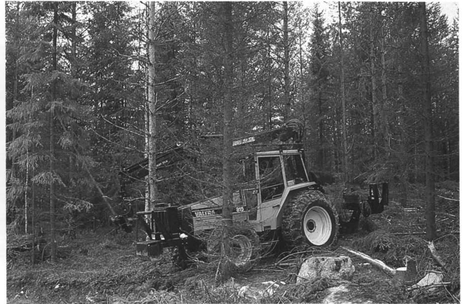
Figure 21. Farm tractors are used increasingly as prime movers for multi-function machines. Valmet 815 farm tractor equipped with Joutsa 46 TX crane and PIKA 36 double-grip harvester (Photo H. Kalaja).
