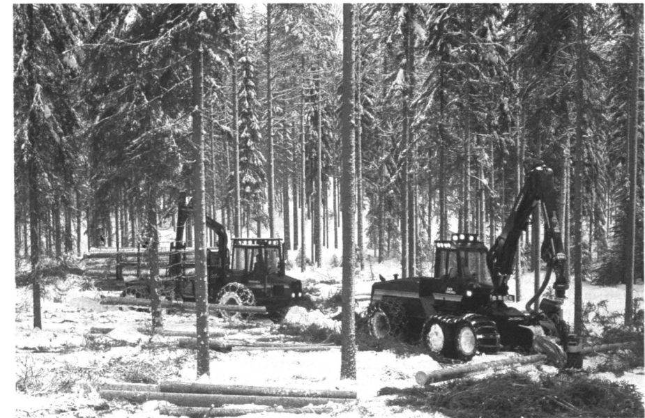
Figure 29. The basic solution for fully mechanized logging is a combination of a single-grip harvester and a forwarder equipped with a long-reach crane. Lokomo 990 single-grip harvester and Lokomo 910 forwarder (Photo FMG Lokomo Forest Oy).
