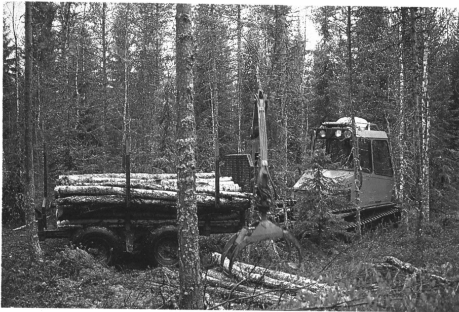
Figure 4. Harvesting small-sized timber from drained peatlands requires special equipment. Forwarding with light rubber-tracked Falmi-Trac crawler (Photo H. Kalaja).
