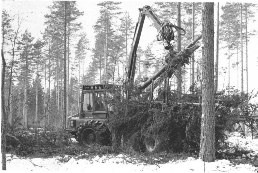
Figure 23. In the tree-section method pulpwood is delivered to the mill with branches intact, whereupon it is delimiting and debarked simultaneously in drums (Photo Erkki Oksanen).
