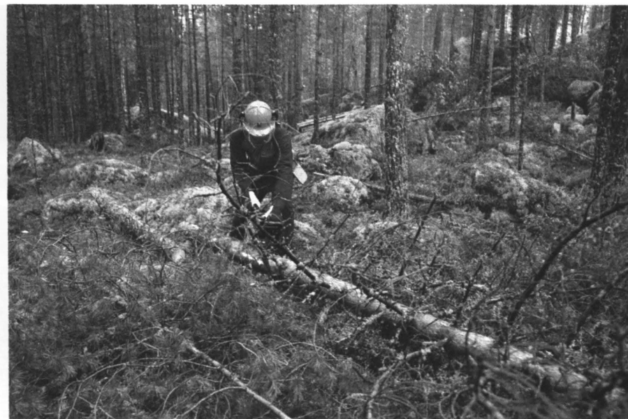
Figure 17. In motor-manual methods, the cutter fells, delimits and bucks the trees. Small-sized pulpwood logs are also bunched (Photo H. Kalaja).
