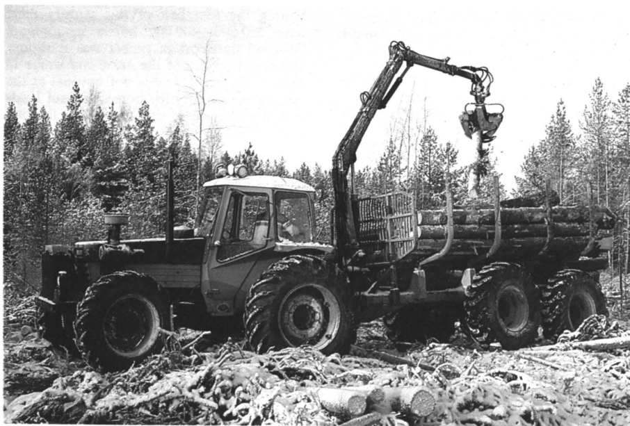
Figure 10. Valmet 903 farm tractor equipped with a self-powered trailer and the RKP 2600 crane for forwarding timber (Photo H. Kalaja).
