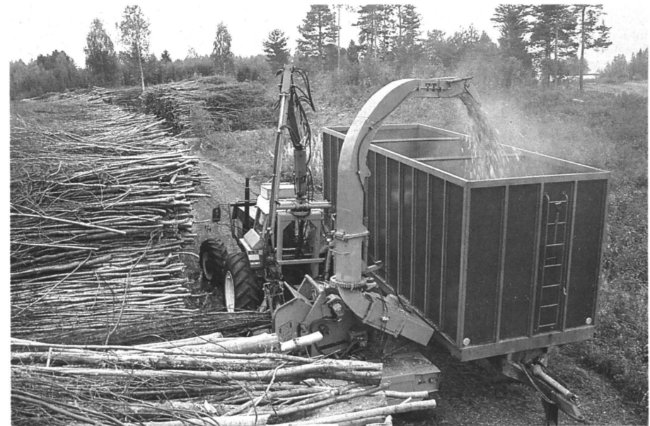
Figure 22. Farm tractors are well suited as prime movers of light and medium-sized chippers for producing fuel chips from small-sized trees. Valmet 903 farm tractor and TT 1000 TU disc chipper (Photo H. Kalaja).
