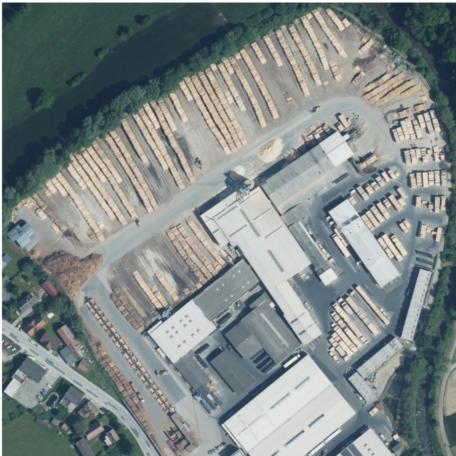
Fig. 5. Log yard layout of the sawmill investigated with a sorting line on the bottom left corner with 40 ejection boxes, storage areas located at the upper left corner alongside a tree line where the debarked logs are stored and the material charge on the top right corner of picture, © GIS Steiermark, 2017, www.gis.steiermark.at .
