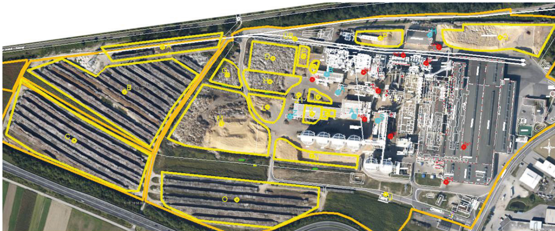
Fig. 7. Layout and storage assignment of sample chip board industry with storage areas indicated in yellow for different geometries of raw material, locations of material charges in turquoise and locations where recycling material accrues in red.
