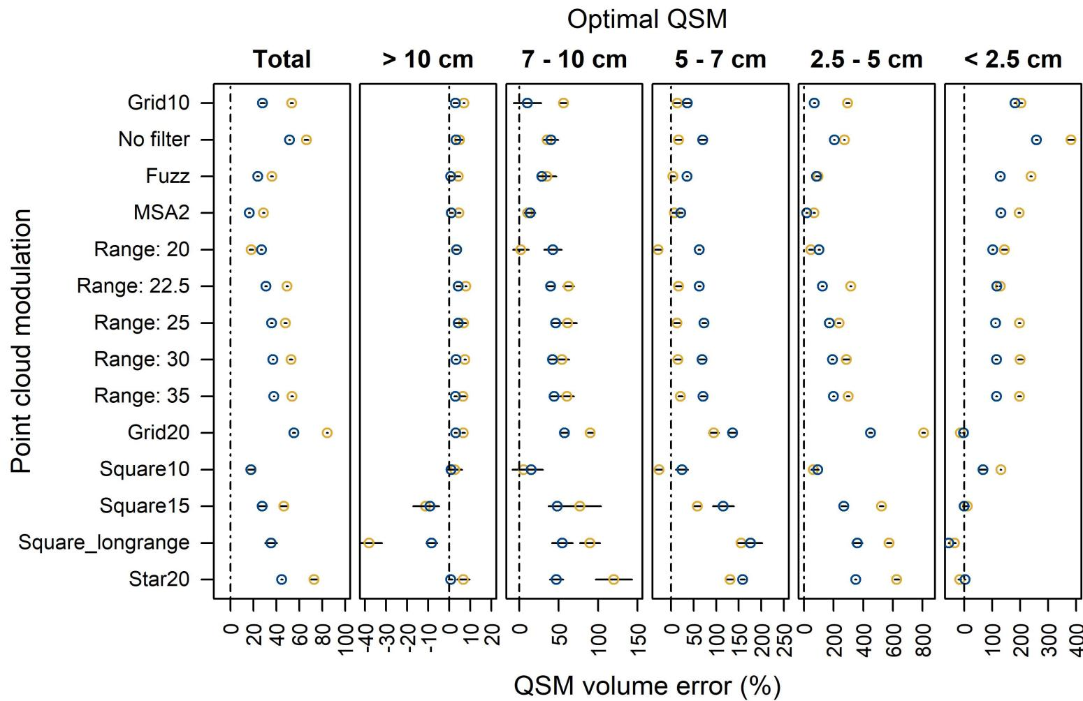
Comparison of QSM volume (points and whiskers) against destructively measured volume (dashed line) in 5 diameter classes for 14 different scanning modulations. Ash #1 in yellow, ash #2 in blue.
