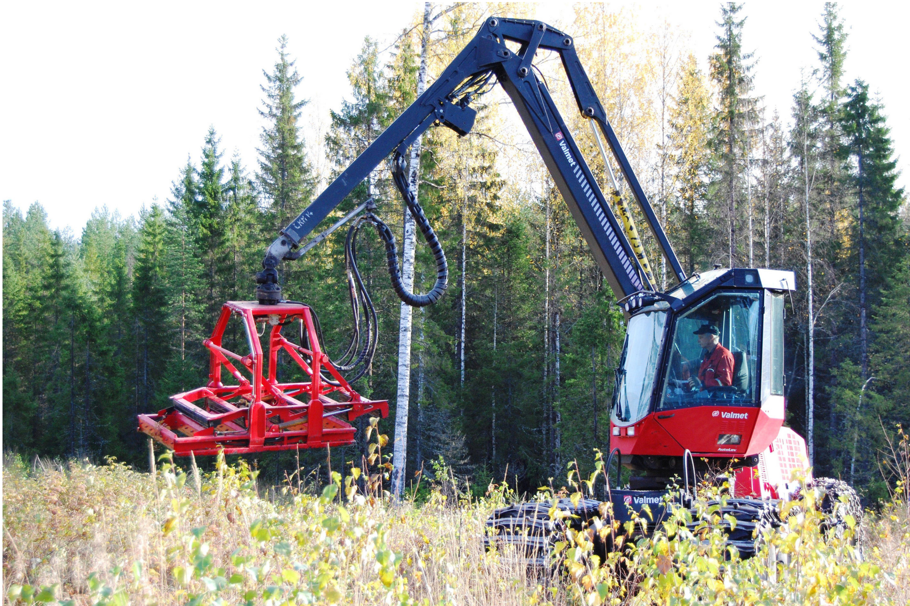
Uprooting device (P25_v1) attached to harvester (Photo: Heidi Hallongren)
